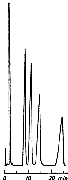
Fig. 2. Analytical chromatogram of glycerol acetal isomers (cf. experimental part).
